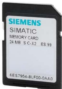
SIMATIC S7, MEMORY CARD FOR S7-1X00 CPU/SINAMICS, 3,3 V FLASH, 24 MBYTE
