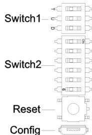
Switch1: DIP switch used to set the terminal resistance, pull up and down resistance. T: terminal resistance, U: pull up resistance, D: pull down resistance.
