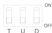
The Switch2: DIP switch used to set the adapter module address. It is set by an 8-bit binary hardware dial - code switch, and each Modbus adapter has a unique station address (1~63).
