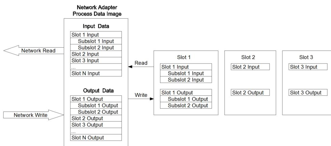
Modbus address mapping table varies according to module combination, and detailed address mapping table could be viewed through IO Config – the configuration software.
