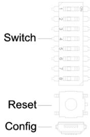
Switch: the DIP switch is used for setting the IP address (the default IP address is 192.168.1.100).
