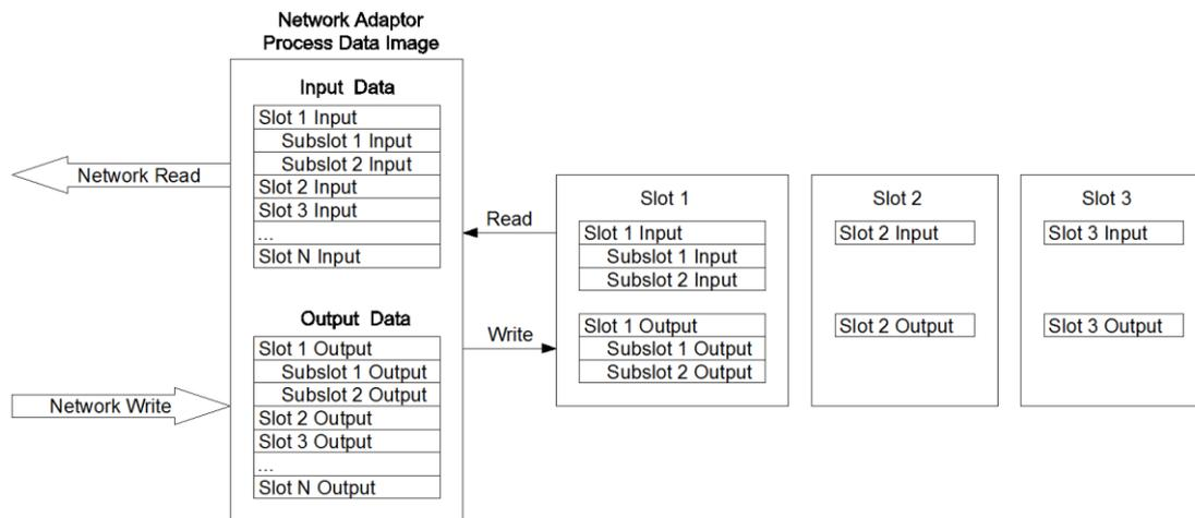
Modbus address mapping table varies according to module combination, and the I/O module address mapping table carried by CN-8031 has two modes.
